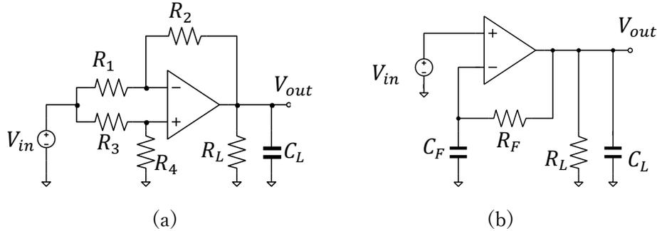
図 1：評価回路 ( $R_1 = R_3 = R_4 = 1k\Omega$ ,  $R_2 = 21k\Omega$ ,  $R_F = 1T\Omega$ ,  $C_F = 10mF$ ,  $R_L = 10k\Omega$ ,  $C_L = 1nF$ )
